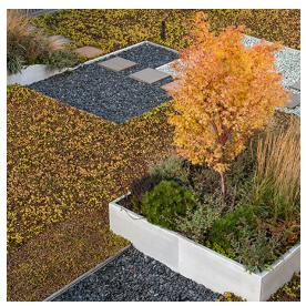
requirements for plant material selected, structural requirements, and stormwater retention goals. Depths typically range from 5" to 8". Consult with structural engineer to ensure your building accommodates the saturated weight of system.
