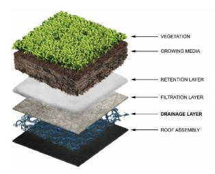
The Drainage Layer does not support mold. Installation is simple and straight forward, involving only heavy duty scissors to cut to shape. The rolls are placed on top of the root barrier or protective sheet and abutted together.
