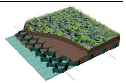
The Sloped Layered system is designed to detain and retain rain and irrigation water, allow hydration of plants, prevent root rot, allow airflow under and up through the multilayer system, allow phyto-remediation (removal of contaminates) from the growing media de-energize wind flow under the multilayer reducing chance of wind uplift, protect the roof with a sacrificial layer under the system and above the waterproof membrane.
